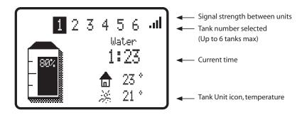
If the Display Unit is not connected to a Tank Unit or is out of range, you will get the message "Disconnected" on the screen when you have selected that tank. If you need to repair a Tank Unit, see (1).
